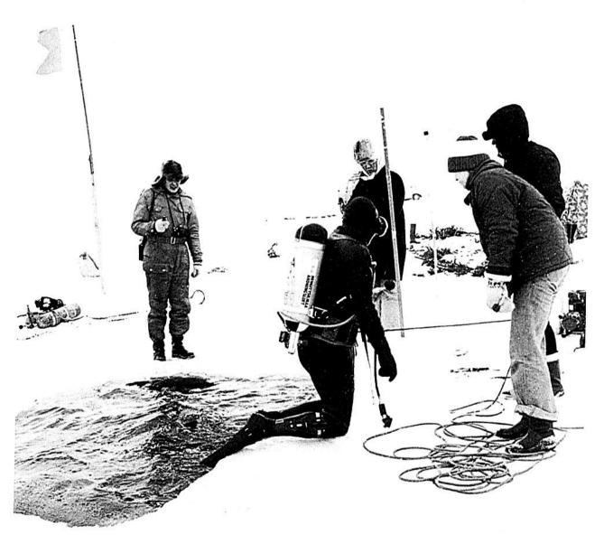
measuring tape/plumbline descending from a float. The rod, kept korizontally by the level, is maneuvred by a diving assistant. One end of the rod touches the initial fixpoint while bearing over the mark in question, where the floating ballasted measuring-tape is brought in to cross the rod. The difference is then easily read.
