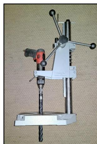
*Picture 5 & 6. MAS volunteer diver using the 4<sup>th</sup> generation drilling device to collect a bore sample of wood.*
