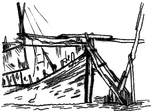
Fig. 5. Aft end of a gajjarije showing the complex steering mechanism. (After Ritter 1919, Abb. 18)
